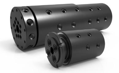
GP models with 2, 3, 4, 6 or 8 flow passages come standard with NPT thread shaft connections and O-ring face seal glands for flush mounting the union to an interface. GPM (metric) models with BSPP connections are not available with O-ring face seal glands.
