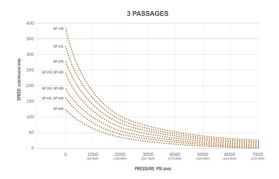
\* This data is to be used as a general guideline. Data based on using hydraulic fluid with the product rotating continuously. Please consult DSTI about your specific application.
