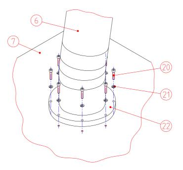
If an extractor arm is used, it is attached by using the flange ring (Pos.22), bolts (Pos.20) and washers (Pos.21) that are provided.
