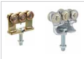
Series -92 double-pair trolley hanger with pendulum hinge of plastic or steel and with counter-pressure roller for sliding leaves with top-hung leaves, height-adjustable
