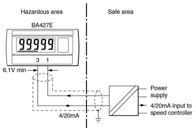
Fig 3 Typical application using a galvanic isolator
