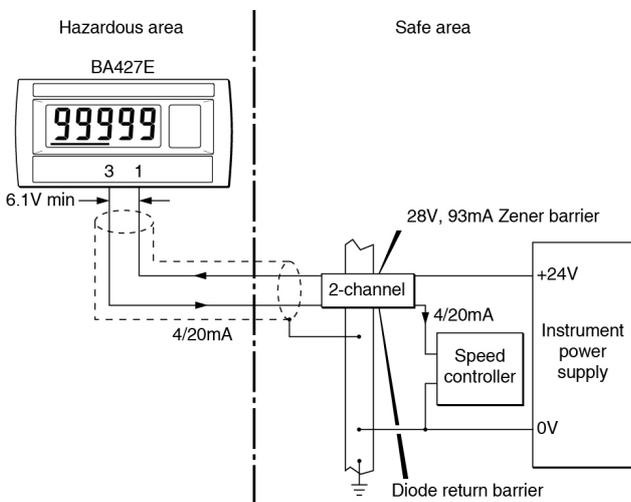
Fig 2 Typical application using barriers
