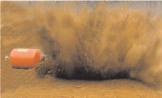
Effect of the isobaric sword nozzle (pat.)
