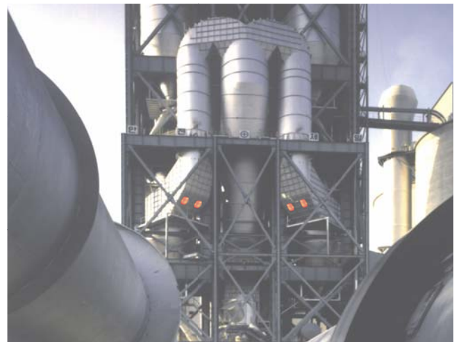
VSR BLASTER® air cannons in a cement plant (Foto: Krupp Polysius)
