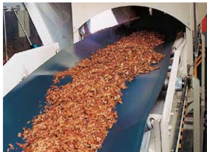
Horizontal conveying with troughable belts. The tension member construction provides the flexibility in the desired direction.
