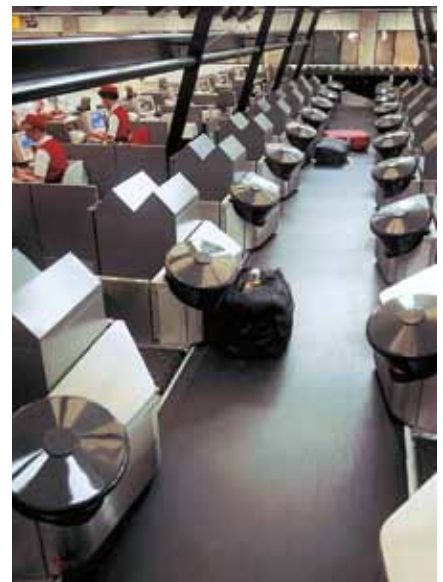
Collecting belt in check-in area of an airport. The flatness of the belt type here ensures that the goods can be discharged to the side smoothly, even on wide belts. Flame-retardance is a "must" in modern airports.
