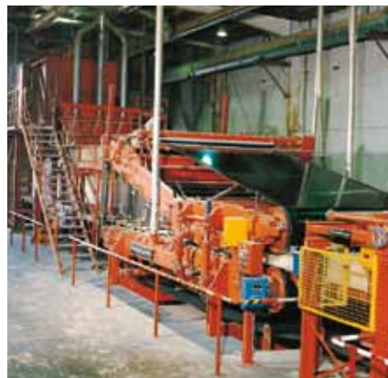
Pre-press belt in the manufacture of particle boards. The particle mat is pre-pressed while being conveyed.
