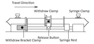
To facilitate loading, the pusher block can be released from the leadscrew by pressing the bronze release button and can be manually moved along the guide rods to accommodate the syringes.
