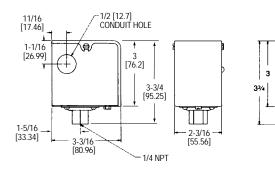
The Series CS Low Cost Diaphragm Pressure Switch is ideal for instrument panels, small compressors and general industrial applications. Visible set point and easy-to-wire SPDT snap switch reduce installation time. This switch operates in any position and is vibration resistant.
