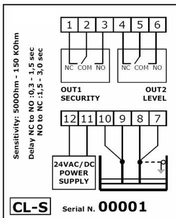
CL-S level switch is capable of checking conductivity between one electrode and a reference electrode.
