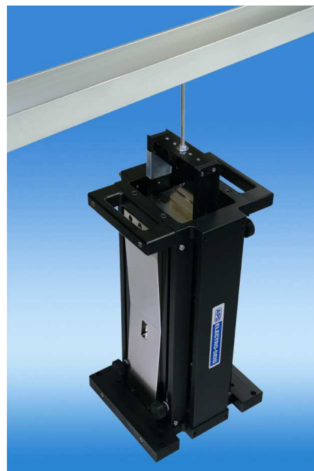
APS 113 with APS 0421 - Carrying Handles and Tie-down Bars and APS 8610 - Connecting Rod prepared for Fixed Body Mode operation
