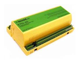
The ETN-40 is a distributed ETN slave module, with 16 optoisolated digital inputs, active at 24 V<sub>DC</sub> or GND, and with 16 relays outputs. It is completely managed by an ETN master controller. The ETN-40 receives the state of the 16 digital outputs from the master controller and sends it back the 16 digital inputs state.
