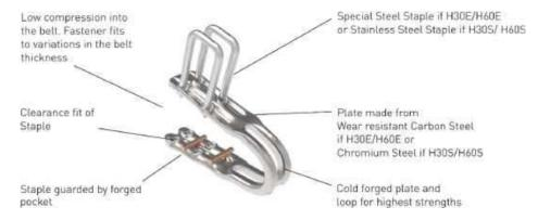
The MR30-System is a simple and easy to use Hammer System. In comparison to other Wide Plate Fasteners, the MR30-System has a long life time and can be installed within a short time.
