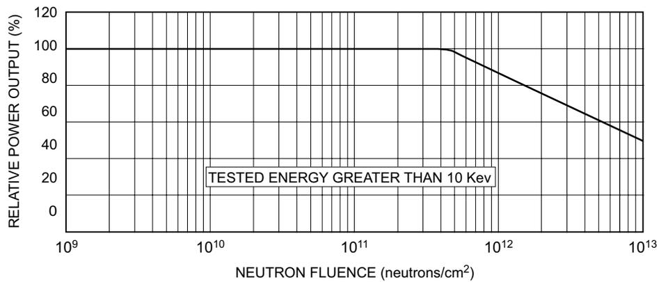
Typical Degradation Curve
