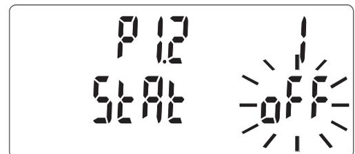
3) Use the [▲] or [▼] key to select "ON", and then press the [ENTER] key. The start date and time setting display appears.
