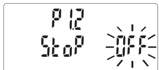
6) Use the [▲] or [▼] key to select "ON", and then press the [ENTER] key. The stop date and time setting display appears. When the preset stop is unnecessary, select "OFF". The preset logging setting screen is resumed.
