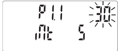
3) Use the [▲] or [▼] key to select the desired logging interval, and then press the [ENTER] key to confirm.
