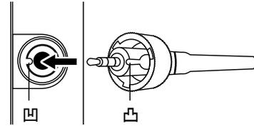
2. Turn the nut clockwise to fasten tightly.
