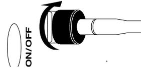
3. To remove the probe, turn the nut counterclockwise to loosen and pull the probe straight toward you.
