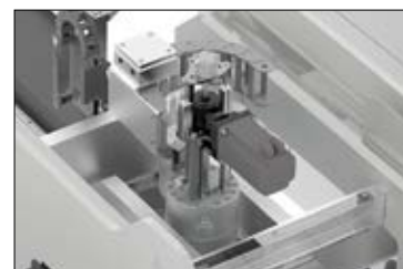
Two-stage punching cylinder • Slow stroke with 600 KN power • Fast stroke with 220 KN power
