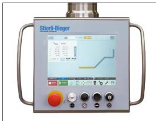
Modern graphic touch-screen control with conversational programming and integrated library of common shapes.
