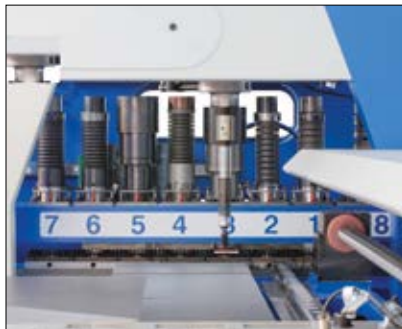
Optional threading from M3 to M16. Three thread diameters can be in operation simultaneously.
