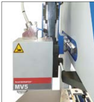
CUProfi and CuMaster marking unit: for labeling of finished parts
