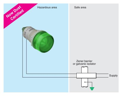
BA390 panel lamps provide reliable cost effective visual status indication in all hazardous gas and dust areas. Each BA390 lamp produces a bright, uniform output with a typical life greater than ten years. All models contain a 20mA current regulator therefore they consume a constant current and hence have a constant brilliance independent of supply voltage. Protection against excess voltage and reverse connection is included in each lamp.
