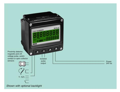
The BA534G is a third generation, general purpose, field mounting rate totaliser housed in a compact IP66 GRP enclosure. The totaliser is easy to use and can be configured on-site to operate with flowmeters having a magnetic pick-off, switch contact, proximity detector, open collector or a voltage pulse output.
