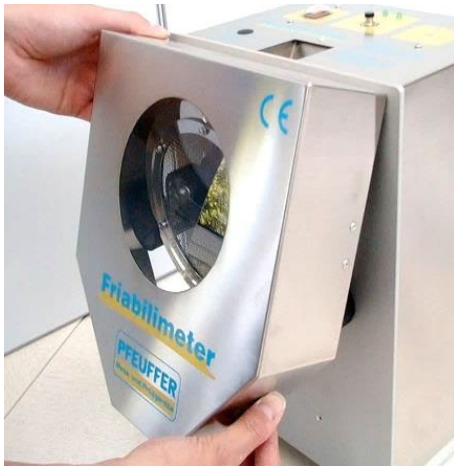
Figure 16: Removing the front cover
