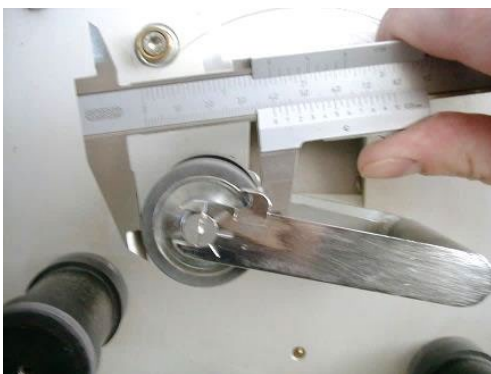
Figure 23: Checking the pressure roll diameter
