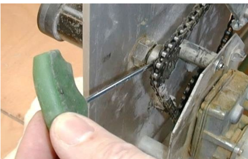
Figure 35: Unscrewing the chain sprocket
