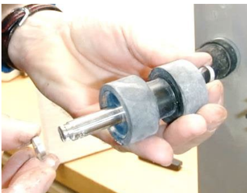
Figure 30: Place spacer rings onto the axle
