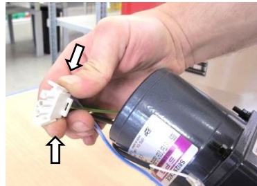
Figure 34: Pressing the motor plug together
