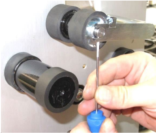
Figure 28: Unscrewing the pressure roll grub screw
