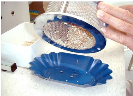
Figure 18: Emptying the content of the sieve drum
