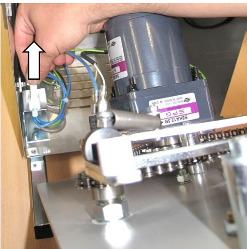
Figure 33: Disconnecting the motor plug
