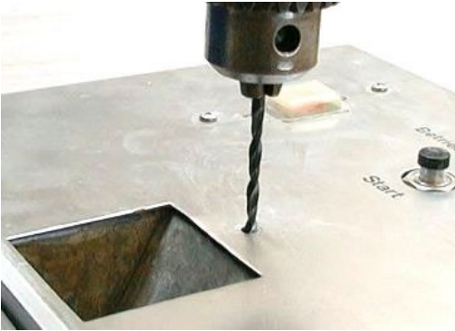
Figure 32: Drilling out rivets
