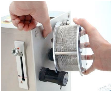
Figure 17: Removing the sieve drum
