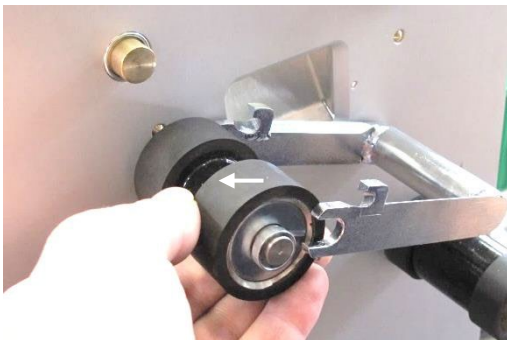
Figure 29: Pulling out the pressure roll
