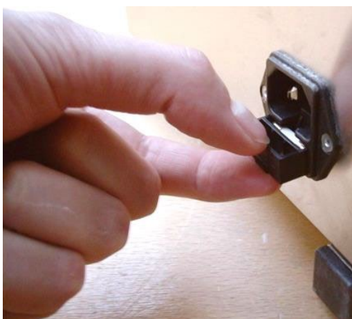
Figure 46: Renewal of the internal fuse
