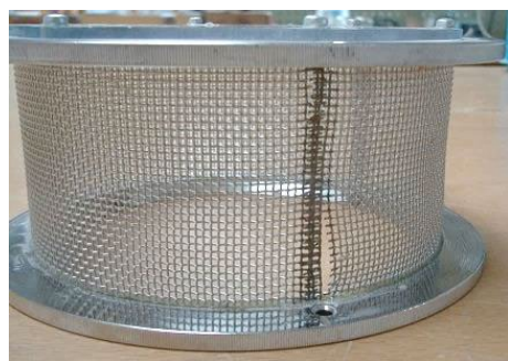
Figure 25: Damaged sieve drum
