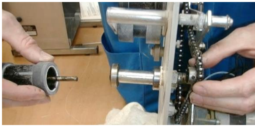
Figure 36: Pulling off the drive roll
