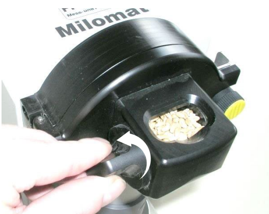
Figure 8: Empty filling hopper
