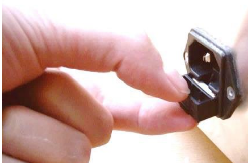
Figure 15: Renewal of the internal fuse
