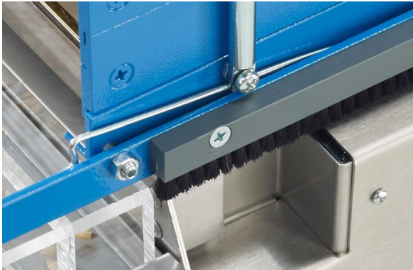
Figure 1: Position of safety spring during operation
