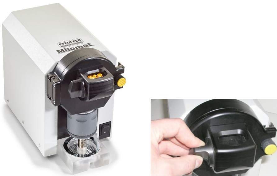
Figure 5: Milomat and measurement cell lower part; turn the dosage button of Milomat
