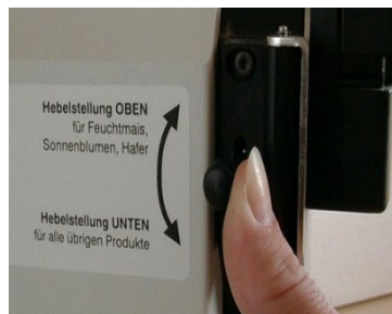
Figure 4: Labomil and measurement cell lower part; adjustment of the lateral lever on the Labomil
