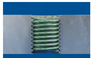
Correct installation of the HELICOIL® Plus ( 0.25-0.5 \times P below the component surface)
