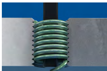
To produce a through-hole thread, the tang is broken off at the notch by means of the tang break-off tool
