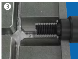
The liquid melted aluminium forced in under high pressure fills the mould and encloses the HELICOIL® Cast on the spindle core without flowing into the internal thread.
