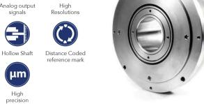
Photoelectric angle encoder A170H is the high end encoder of the product range. It has a hollow shaft and an integrated stator coupling and is capable of producing up to 3.600.000 output pulses per revolution with the accuracy that can reach up to ±2.5 arc. sec.
