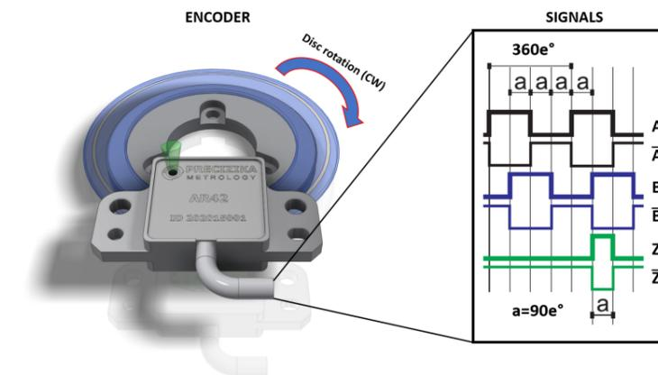
B lags A for clockwise direction (viewing from the top)
