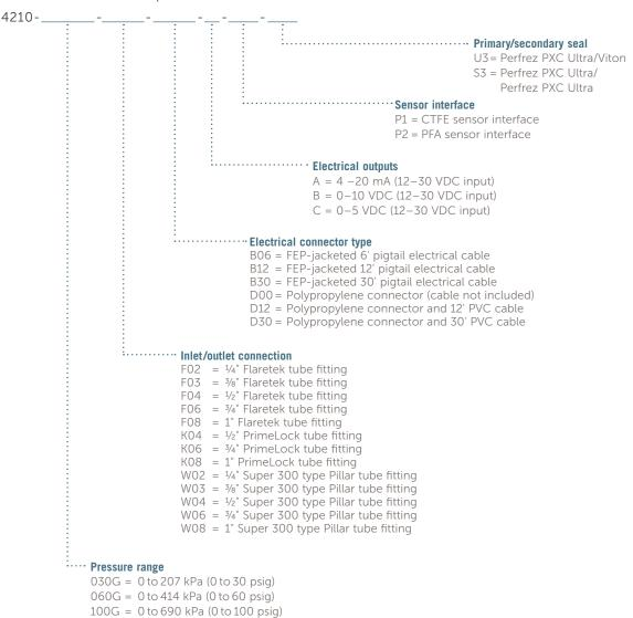
Note: Product specified with a flared connection is packaged with two PVDF nuts. For alternative nut material or custom configurations and specifications, please contact the factory.
