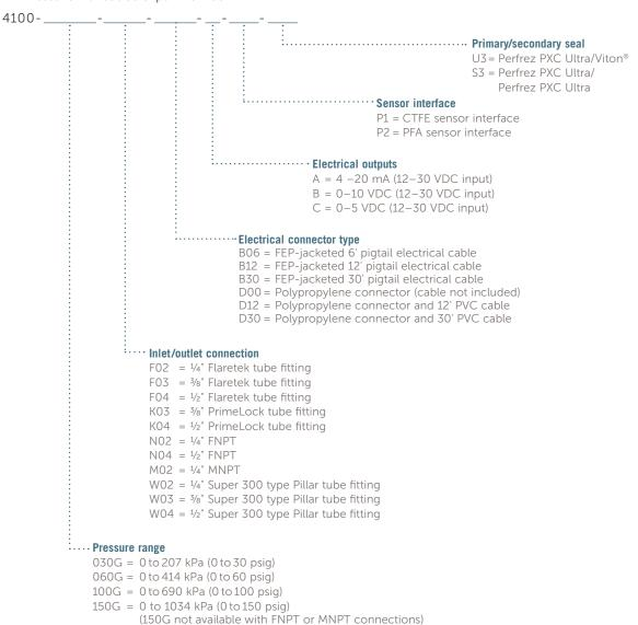
Note: Product specified with a flared connection is packaged with one PVDF nut. For alternative nut material or custom configurations and specifications, please contact the factory.
