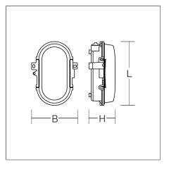
Robust die-cast aluminium LED oval luminaire in flat design. Housing: die-cast aluminium, powder-coated. Diffuser made of textured toughened crystal glass, opal. Diffuser attached with lateral spring clips. Full-surface homogeneous illumination. Suitable for ceiling mounting, wall (surface). Speedy installation thanks to external fastening clips. Replaceable LED unit. Three cable inlets. Suitable for use in harsh environments.
