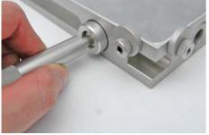
Install the connecting adapter to the stop.
