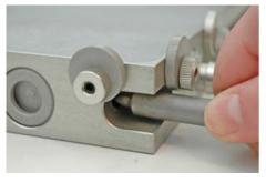
Fig. 4: Release the screws
