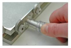
Fig. 3: Connect the vacuum hose
