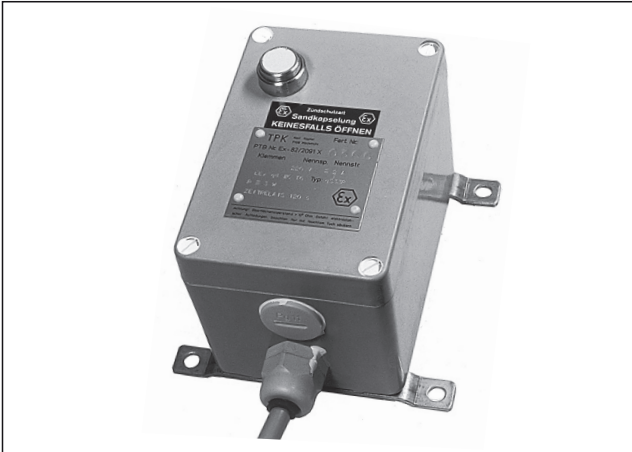
Powder-filling protection with cable ends of a firmly adjusted time relay with a built-in start pushbutton. Polyester housing, 110 x 75 x 75 mm
