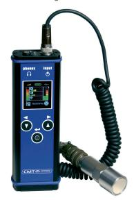
Statistics show that insufficient bearing lubrication is the most common cause for most bearing damages. Using the CMT Vibration Meter to find insufficient lubrication is fast and simple. A single measurement of only a few seconds gives information about the lubrication of the bearing. Avoid bearing damage and unnecessary costs without much effort.
