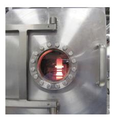
GH Vacuum Furnaces are designed to heat parts of virtually any shape in a high temperature, high vacuum environment or in partial pressure of an inert gas.
