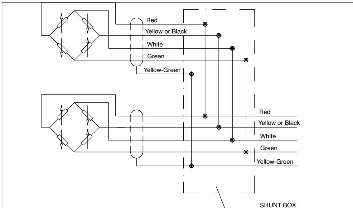
In systems that use several cells, the parallel connection automatically sums the loads on each individual cell.
