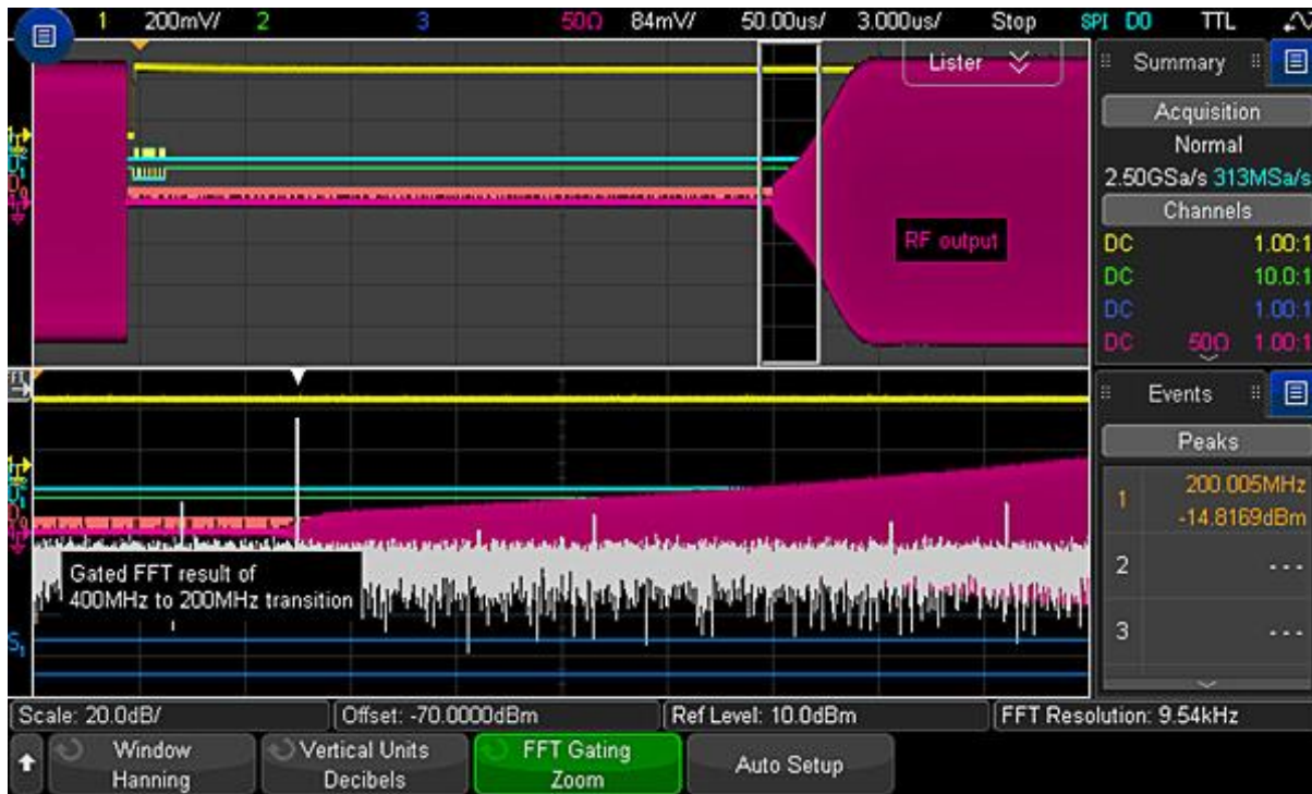
Figure 23. Start observing the RF signal at 200 MHz. You can validate this from the RF analog waveform as well.
