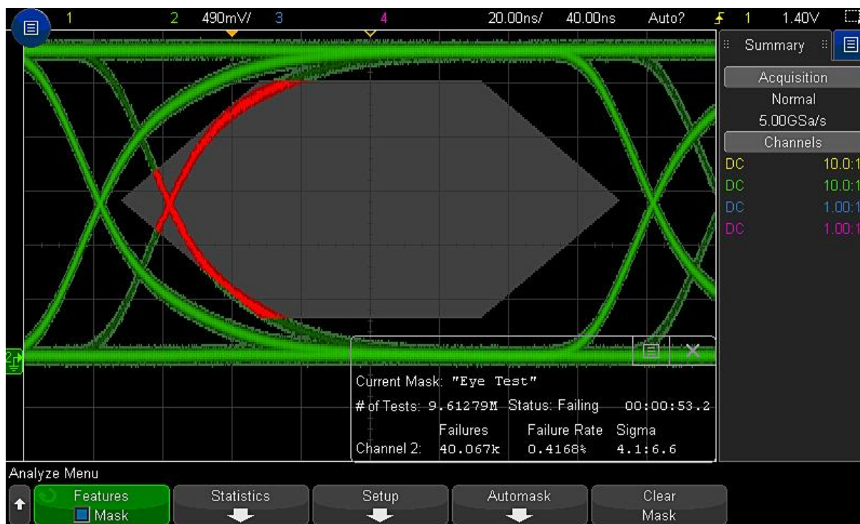
Figure 32. Hardware accelerated mask testing allows testing against a golden waveform or user created mask to find violations. In this example we captured over 9M tests in only 53 seconds.
