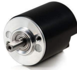
Photoelectric rotary encoder **A28** is a small 28mm diameter incremental encoder that can have up to 25.000 output pulses per revolution.
