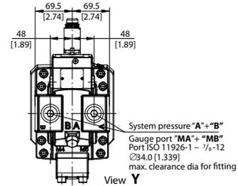
Cartridge with Electric two-position control (de-energized = min. displacement)
