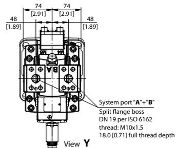
DIN ISO 3019/2 with Electric proportional control (de-energized = min. displacement)
