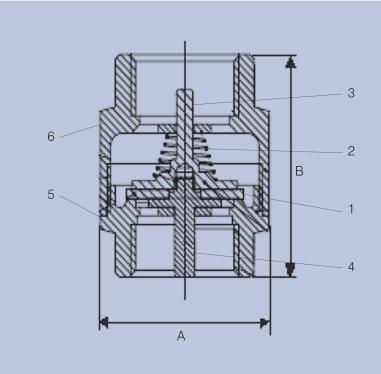
Valve range 1451 Spring Check Non Return Valve - PN10/12 - (Brass)
