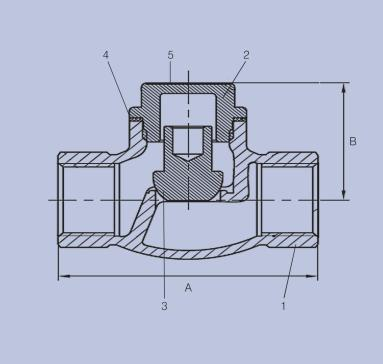
Valve range 1360 Horizontal Lift Check Valve - PN32 - (Bronze)
