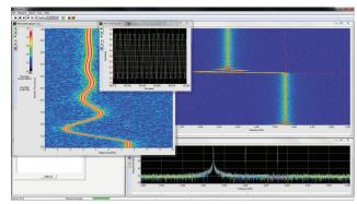
Spectrogram time windows positioned in time and frequency by marker placement.
