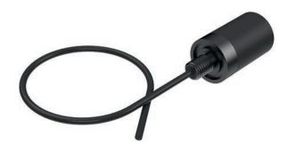
The Model T216 is designed for use in transponders, beacons, acoustic release mechanisms and data communication systems. This versatile transducer combines efficient broadband transmission and reception suited to tracking applications on underwater vehicles and range trials. The anodised aluminium base incorporates a threaded fastening and 'O' ring seal allowing simple and direct mounting onto
