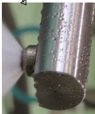
OP nozzle for fine water droplets spray
