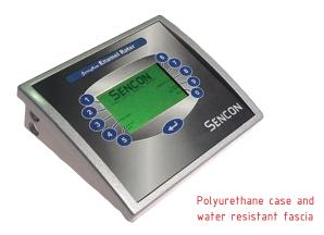
Sencon's Semi-auto Enamel Rater checks lacquer integrity on cans and ends using the industry standard conductivity test. A small, safe voltage is applied between an electrolyte (conductive fluid) inside the can and the body of the can. The amount of resultant current flow indicates the amount of metal exposure caused by any imperfections in the lacquer.
