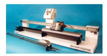
The system consists of two specialized non-contacting End Count Sensors that are designed to achieve reliable and highly accurate counts to allow precise monitoring with 100% confidence. The sensors are positioned on a carriage mounted to a linear bearing, which allows the stack to be easily and swiftly moved past the counter. The ends are counted in 'stick' form, which
