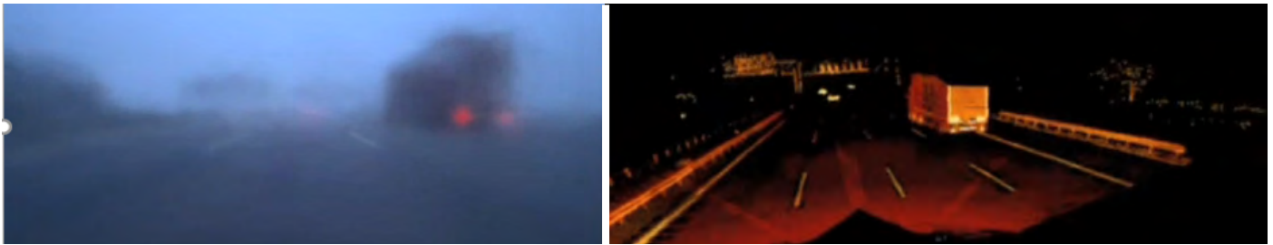
Figure 8: Camera vs. LiDAR in mist/rain
