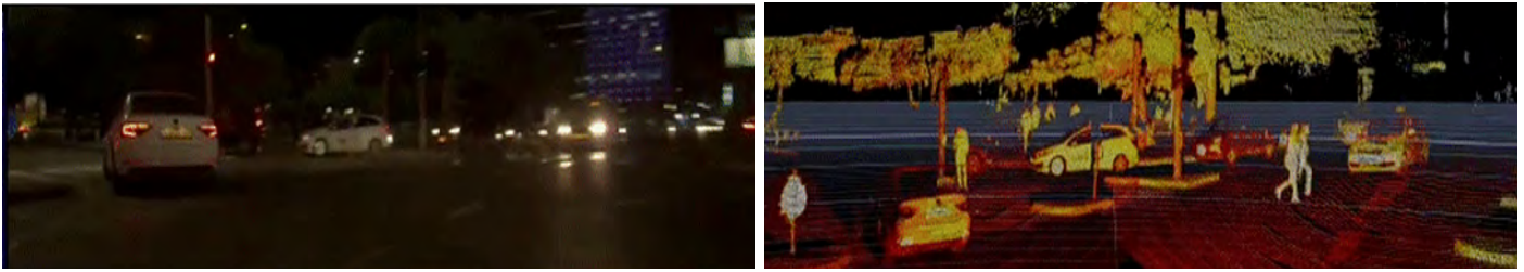
Figure 7: Camera vs. LiDAR in low-light conditions
