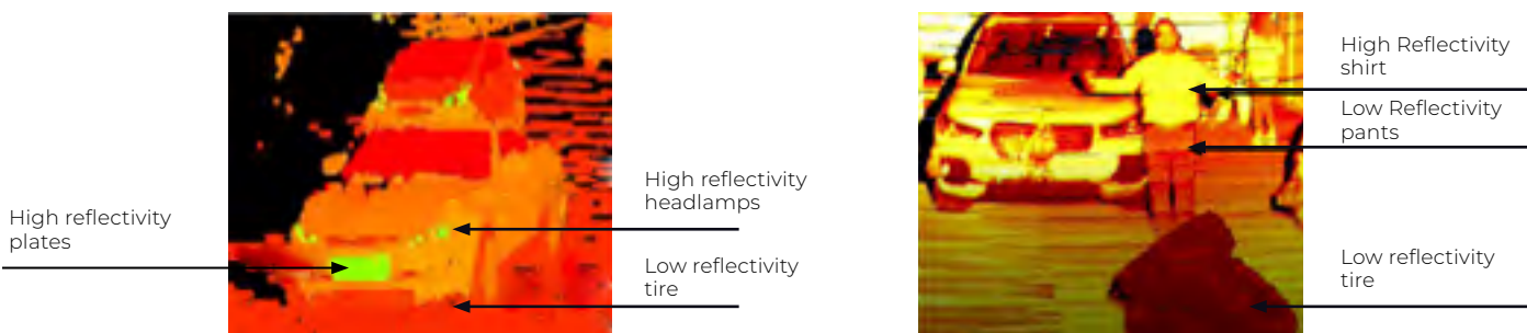
Figure 34: Point cloud detection of various reflectivities
