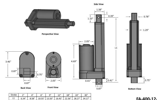
\*Stroke length tolerance: ±0.125"
