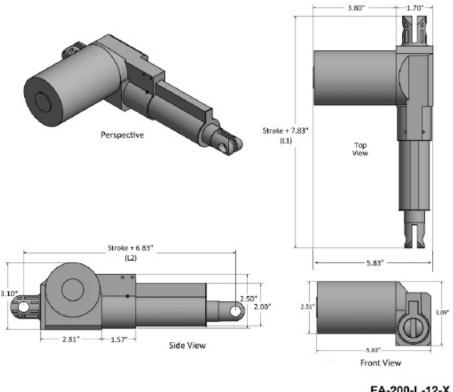
\*Stroke length tolerance  $\pm 0.125^{\circ}$
