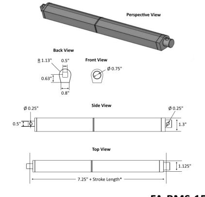
\*Stroke length tolerance = ±0.125"
