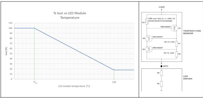
The thermal measurement is performed connecting NTC circuit from the pin LED+ and the NTC pin.
