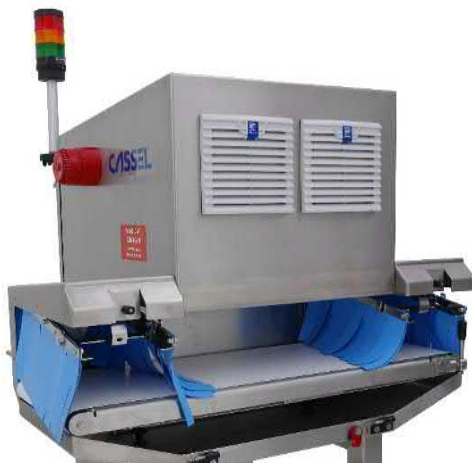
Removable double curtains for user protection and easy handling.
