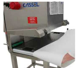
Remove conveyor belt.
