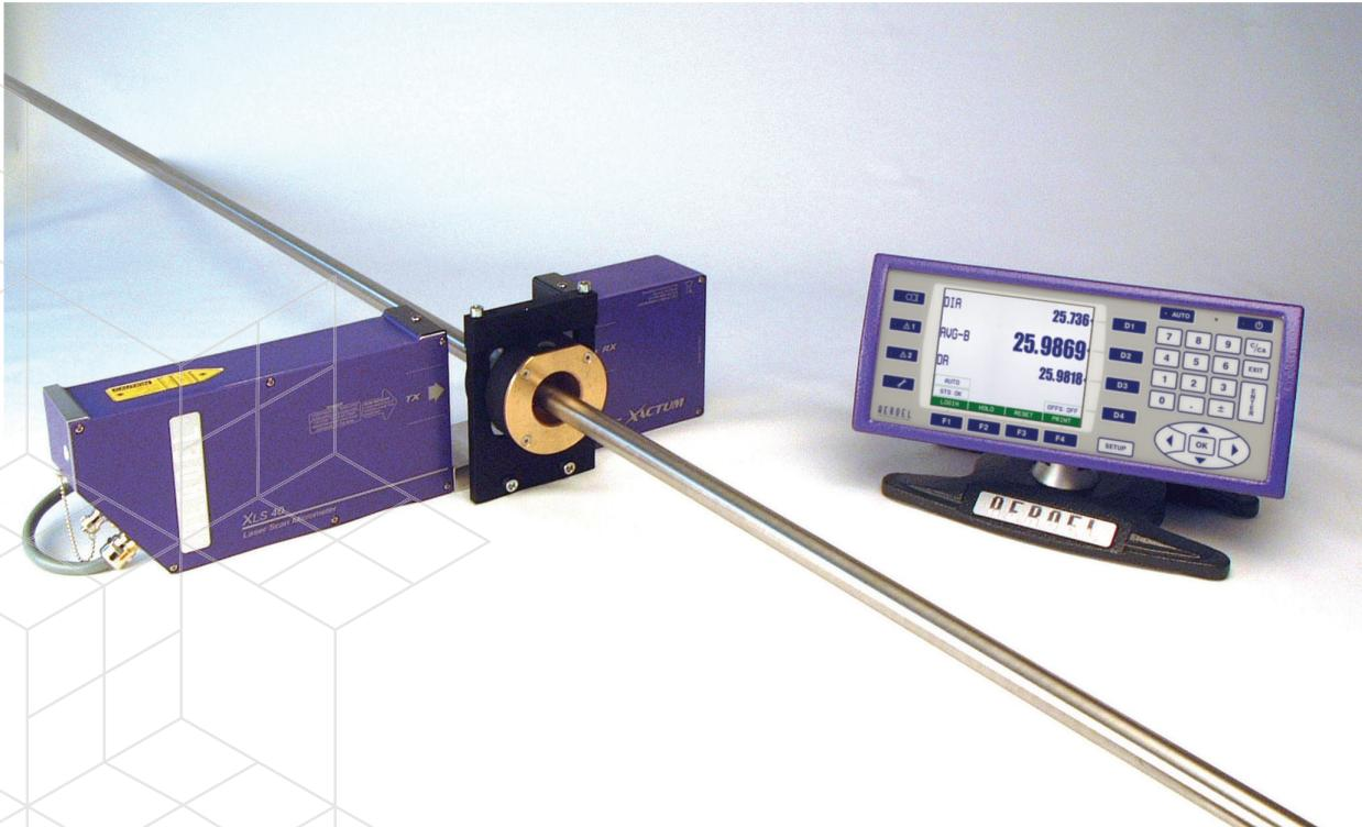
The Barline.X Laser System has been specially designed for on-line gauging of the outside diameter of products manufactured in cut lengths; such as steel ground bars, steel drawn tubes, copper tubing, etc.
