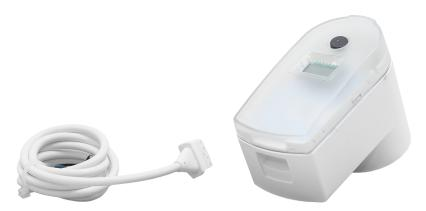
The motorized valve actuators are designed for applications that need short response time for the valve control. The actuators are equipped with removable cable (1 m) and they are available for 3-point control and 0...10 V control. An adapter between the valve and the actuator is always needed.
