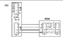
Wiring Example: RDM connected to RSH-24V-R using the Remote Strobe/Horn Terminal
